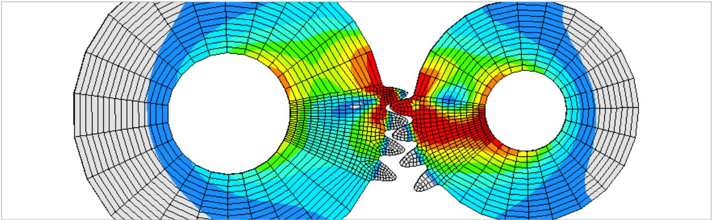
Von Mises stress plot of gears using a sliding contact
